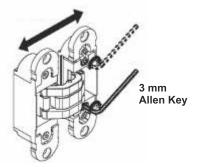
Adjusting the Z axis - door panel up/down
