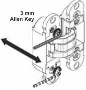
Adjusting the Y axis - door panel in/out
