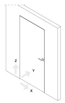
Adjusting the X axis - door panel right/left
